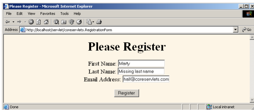
Figure 8–12 When the input form is incompletely filled in (top), the RegistrationServlet redirects the user to the RegistrationForm (bottom). The RegistrationForm uses cookies to determine the values of the form fields that were already filled in.
