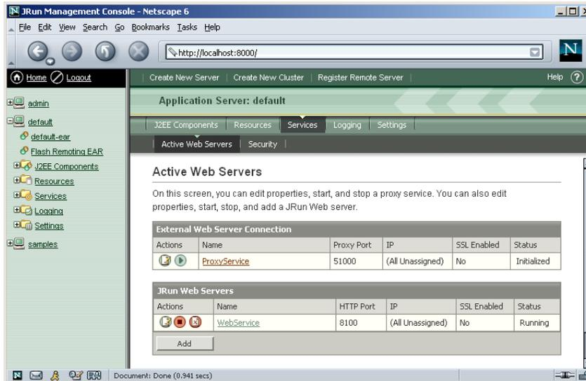
**Figure 2-7** After selecting Services under the default server, choose WebService to edit the port of the default JRun server.
