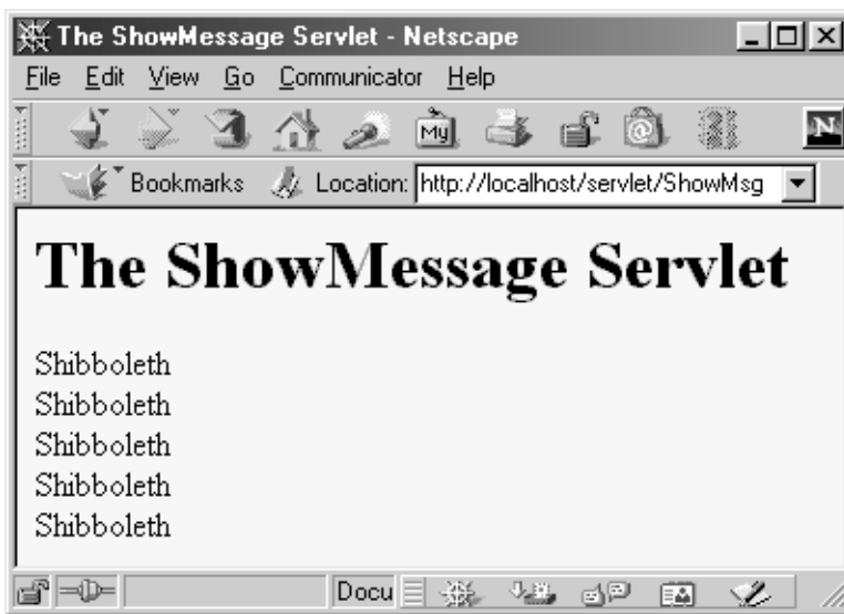
Figure 2-5 The ShowMessage servlet with server-specific initialization parameters.
